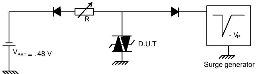
This is a GO-NO GO test which allows to confirm the holding current ( $I_H$ ) level in a functional test circuit.
